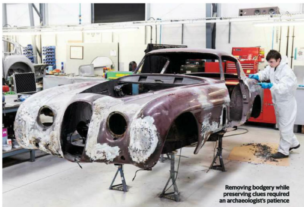
Front sections had to be reformed with fresh steel
