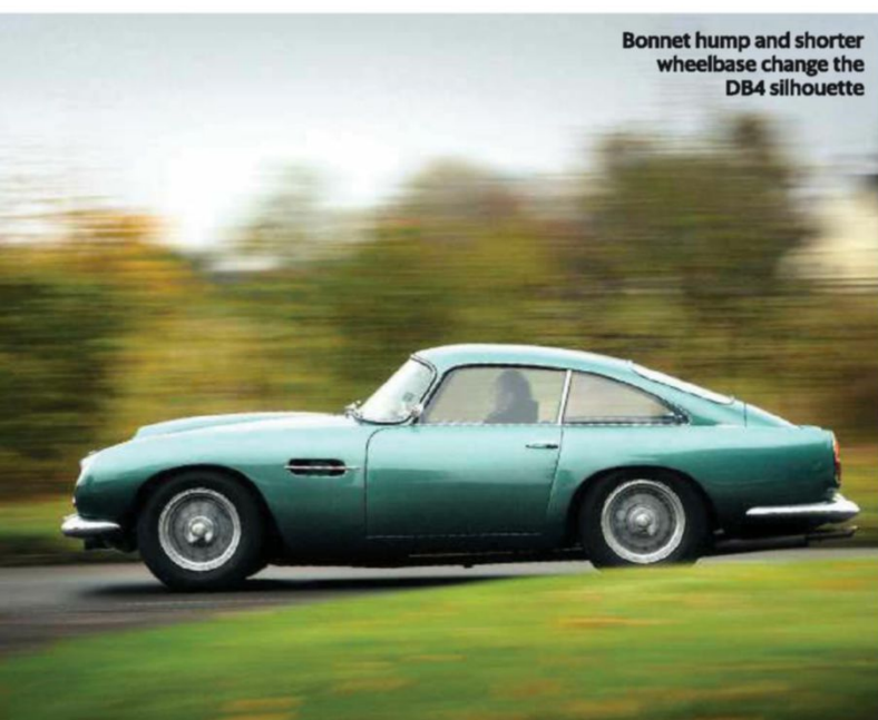
Aston gently coaxed five inches out of the DB4's wheelbase without a negative impact on Carrozzeria Touring's original design
